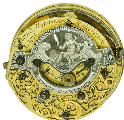
Kent uzelve Know yourself. Motto and associated icon on the silvered 'mock pendulum' balance bridge at the backplate of an early 18th C. Dutch pocket watch.
